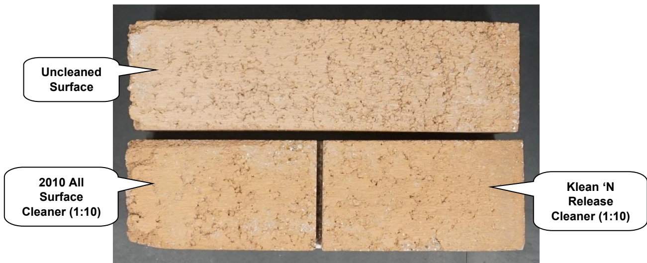
"Adobe" Concrete Brick After Cleaning
