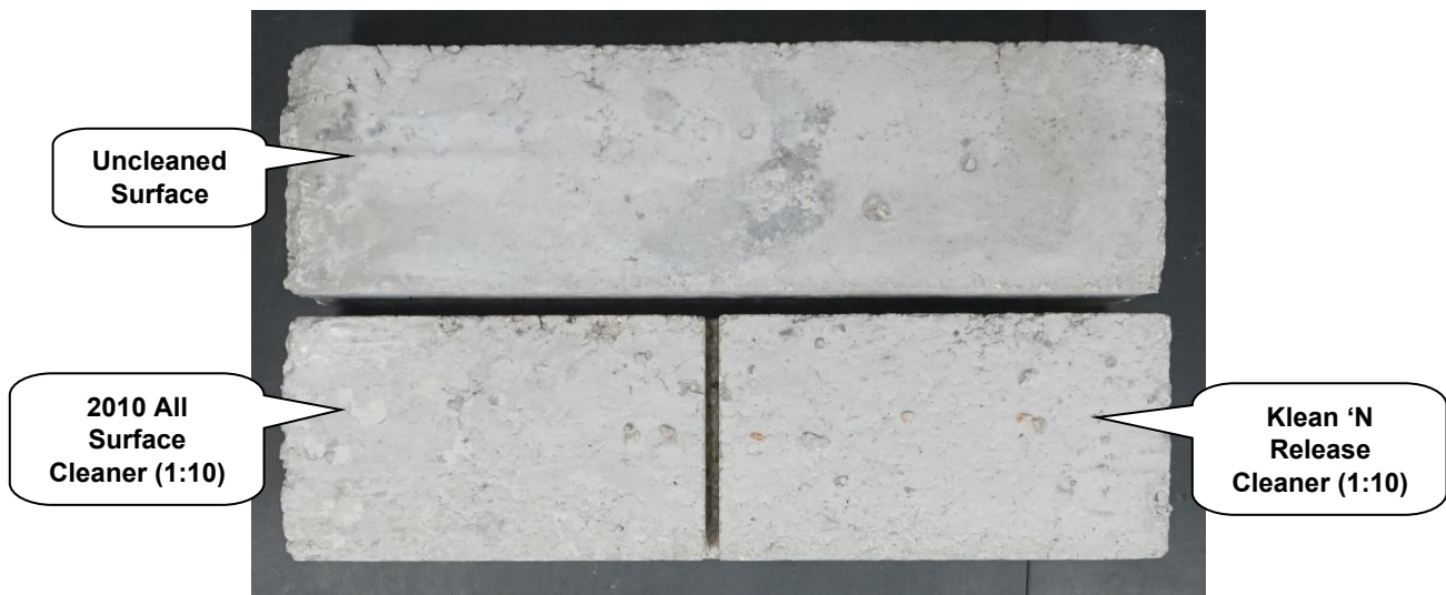
"Dartford" Concrete Brick After Cleaning
