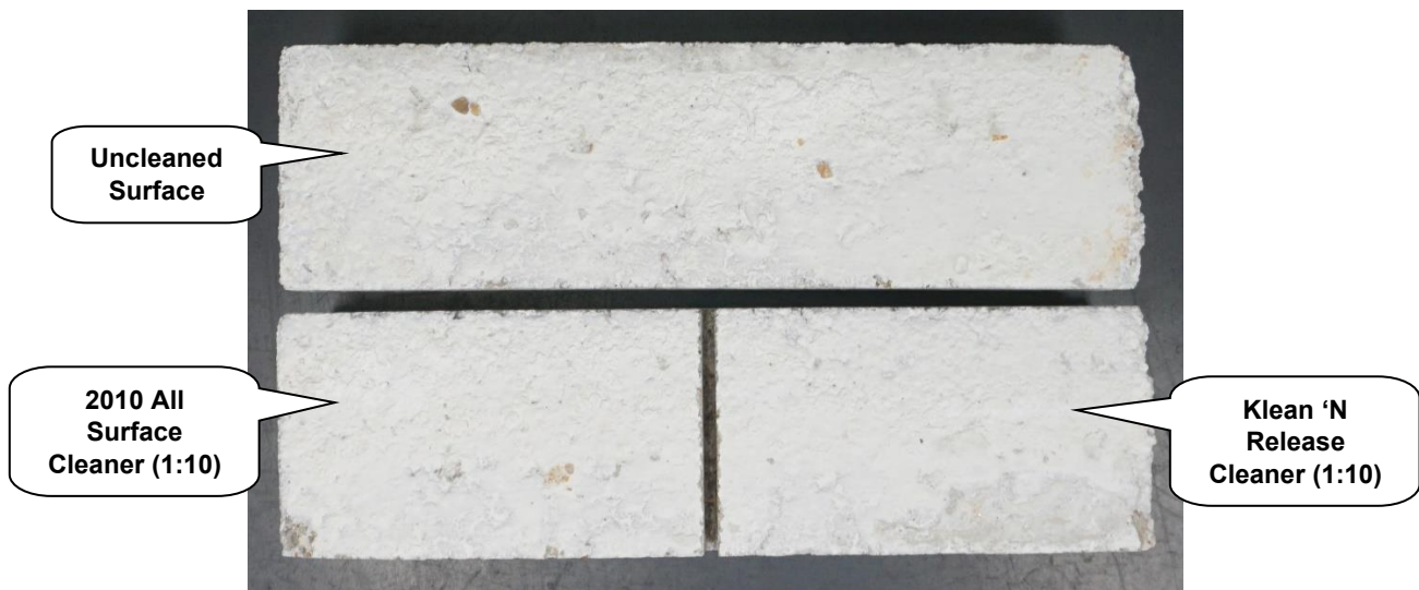
"Everest" Concrete Brick After Cleaning
