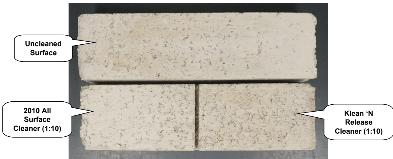
"Dune" Concrete Brick After Cleaning
