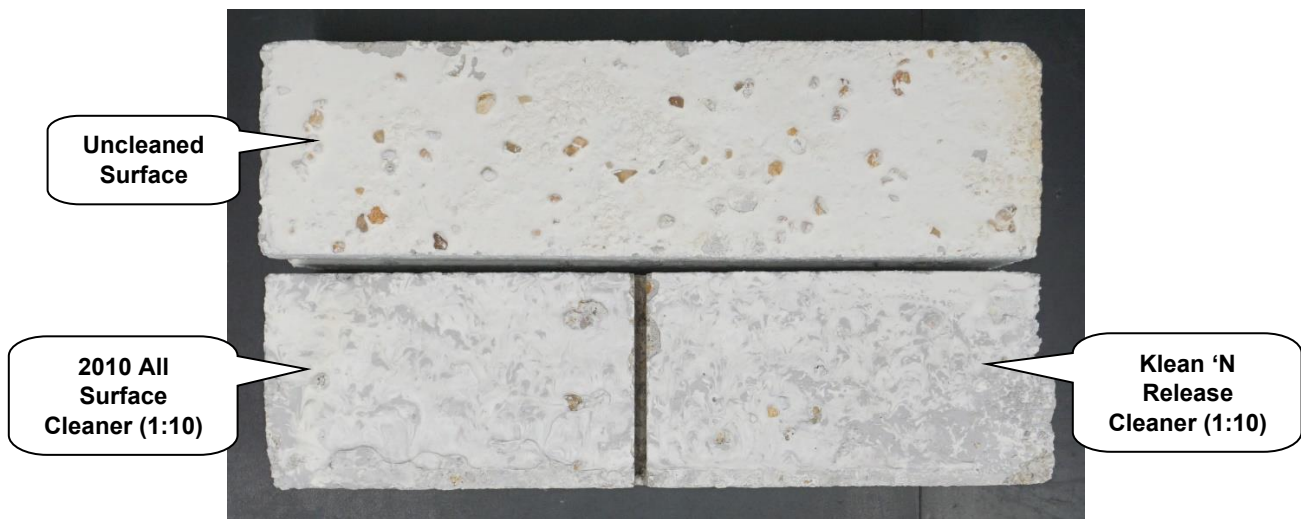
"Winter Ash" Concrete Brick After Cleaning
