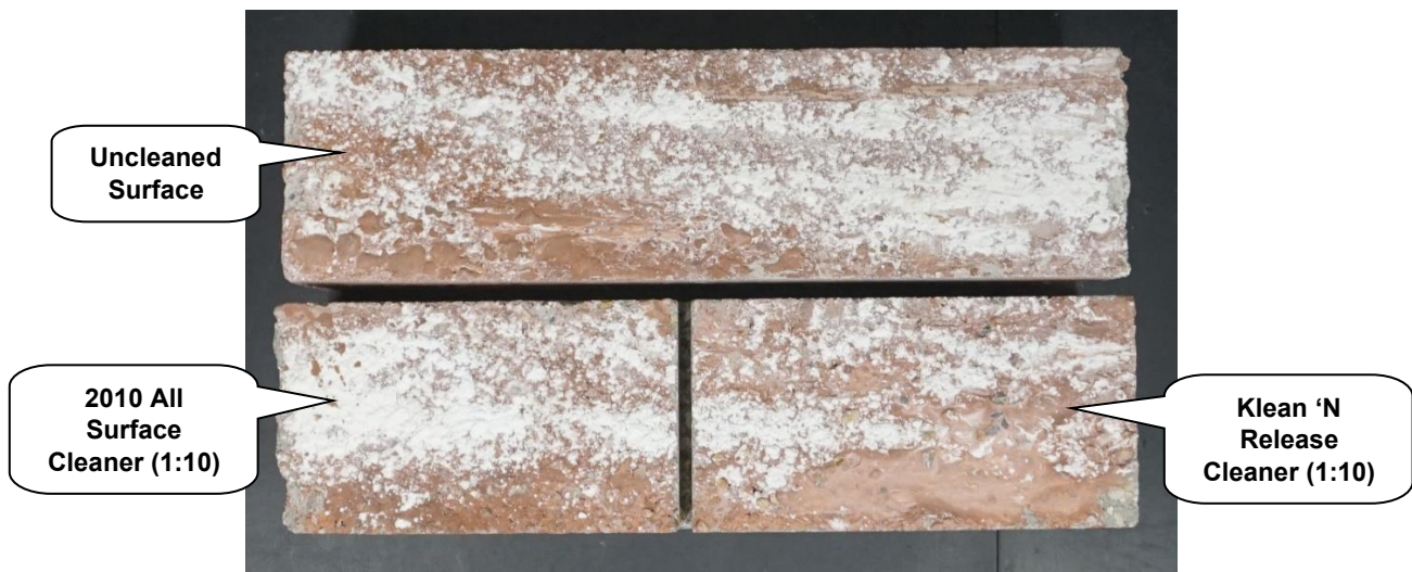
"Williamsburg" Concrete Brick After Cleaning
