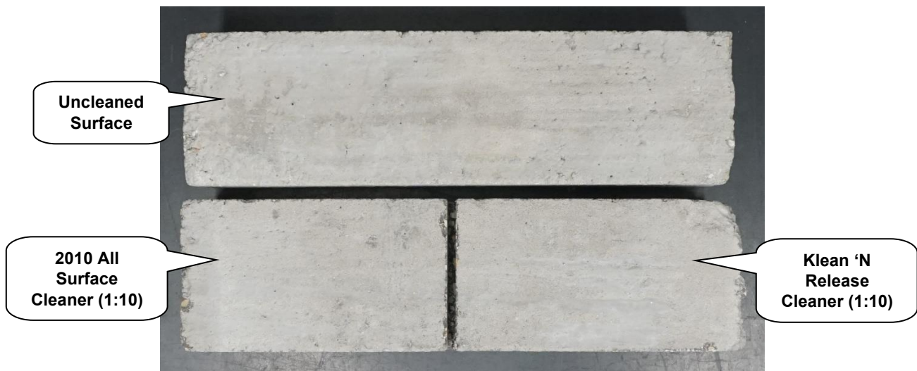
"Gray Mist" Concrete Brick After Cleaning
