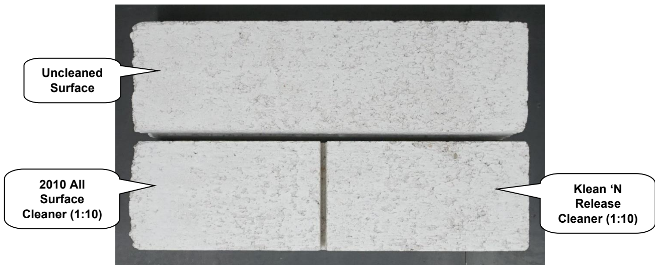
"Phoenix" Concrete Brick After Cleaning
