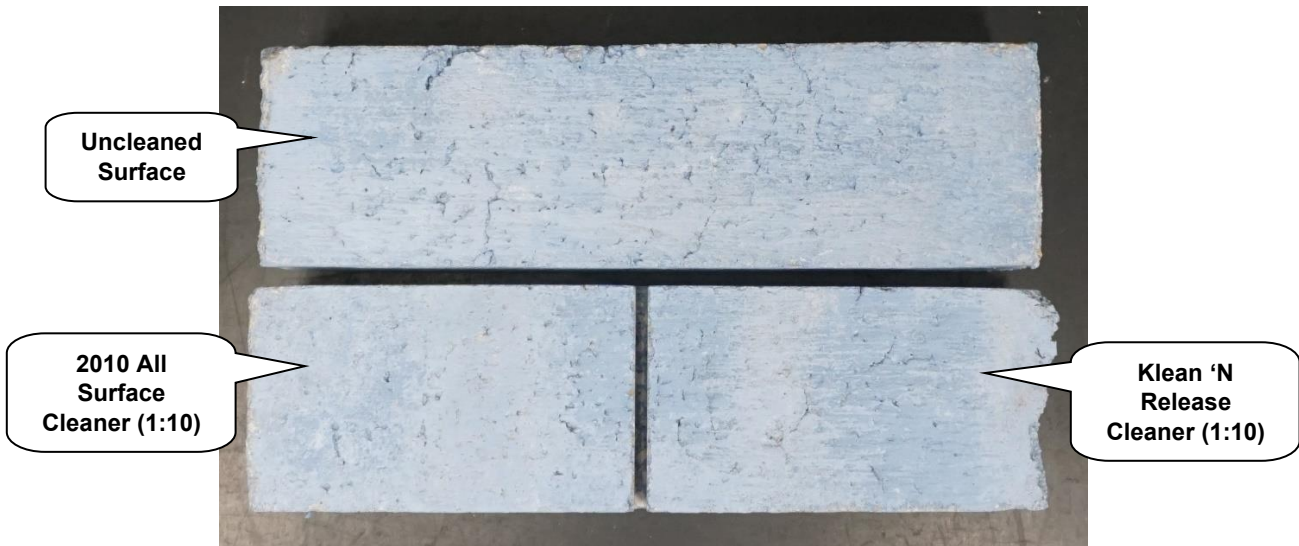
"Caribbean Blue" Concrete Brick After Cleaning
