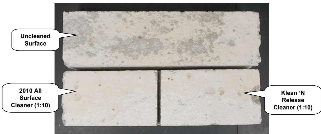
"Bristol" Concrete Brick After Cleaning
