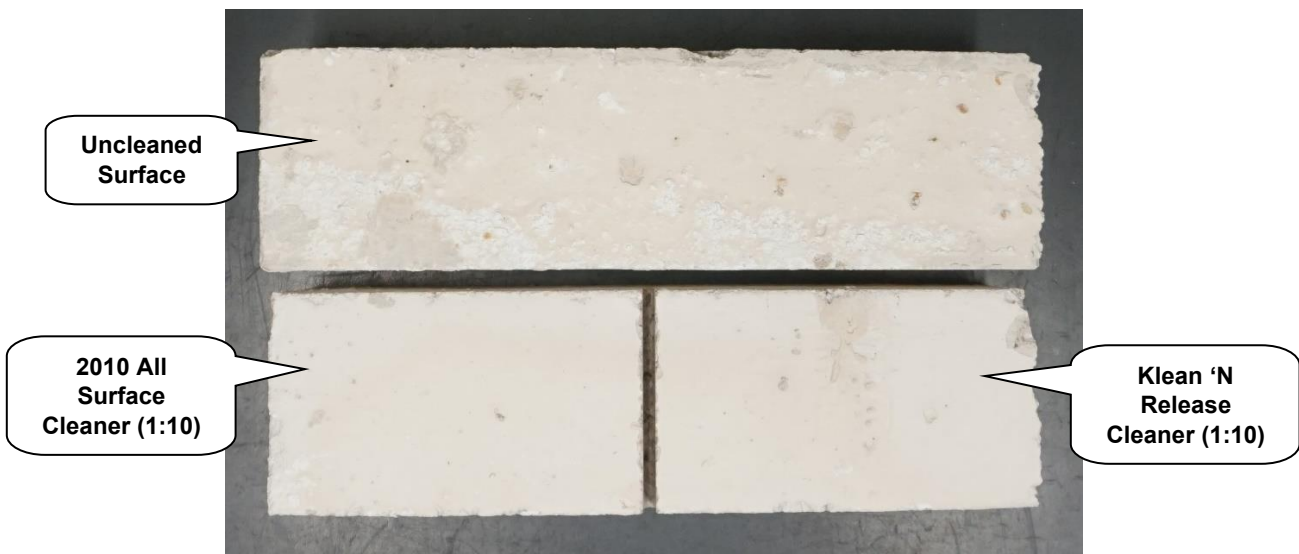
"Wheaton" Concrete Brick After Cleaning
