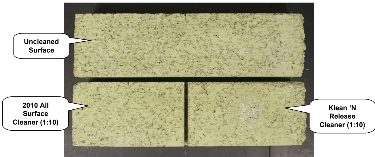
"Lime Green" Concrete Brick After Cleaning
