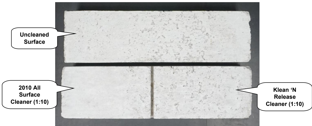
"Mountain Peak" Concrete Brick After Cleaning
