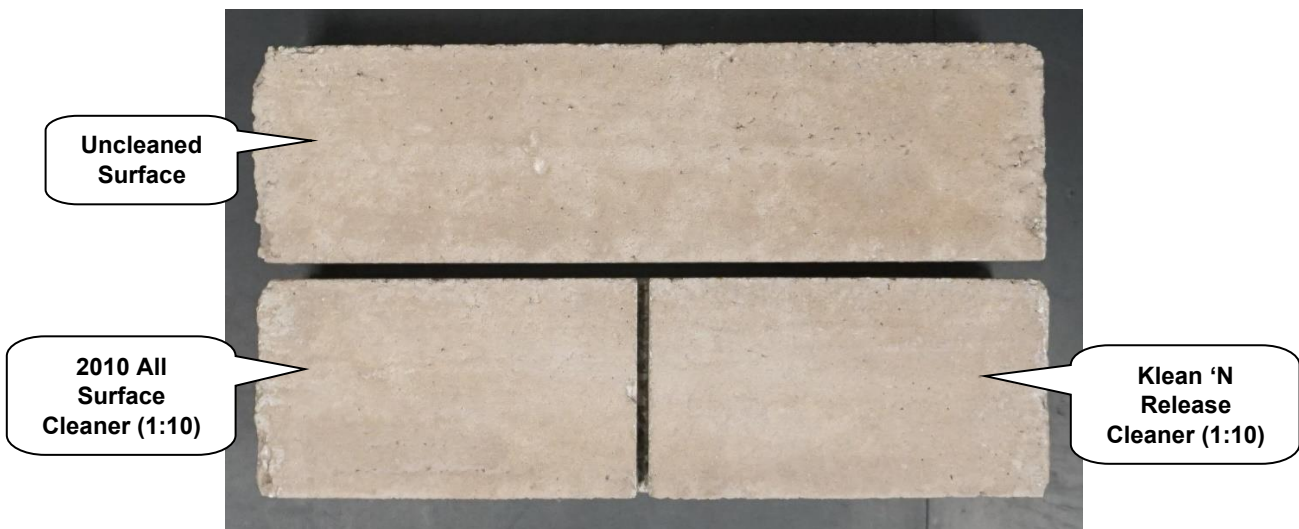
"Chestnut" Concrete Brick After Cleaning
