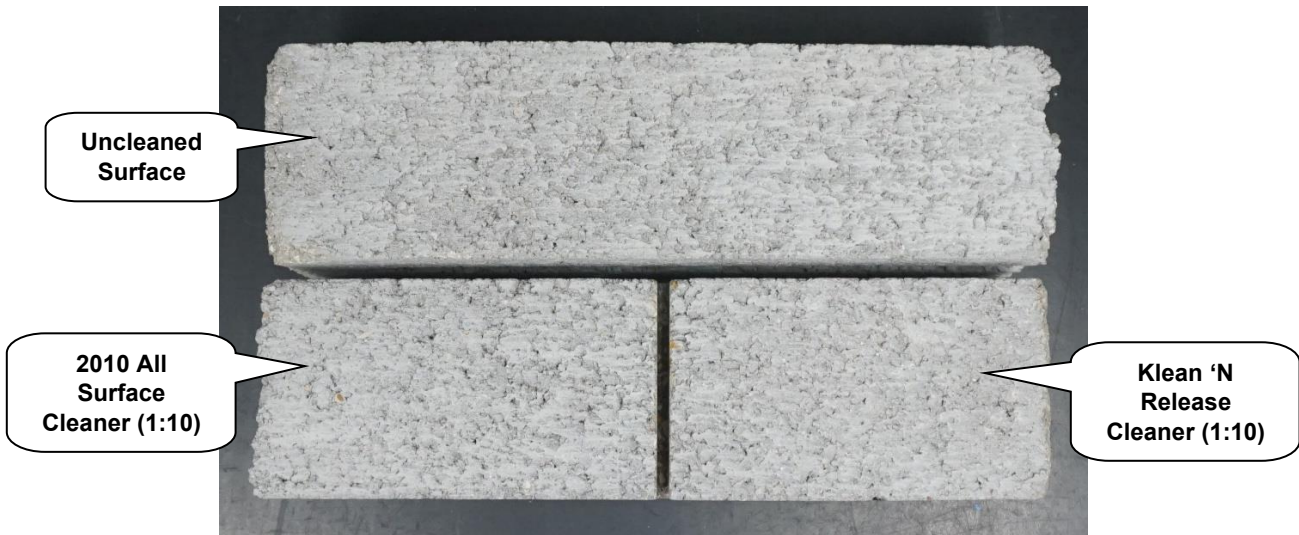
"Bilco Gray" Concrete Brick After Cleaning
