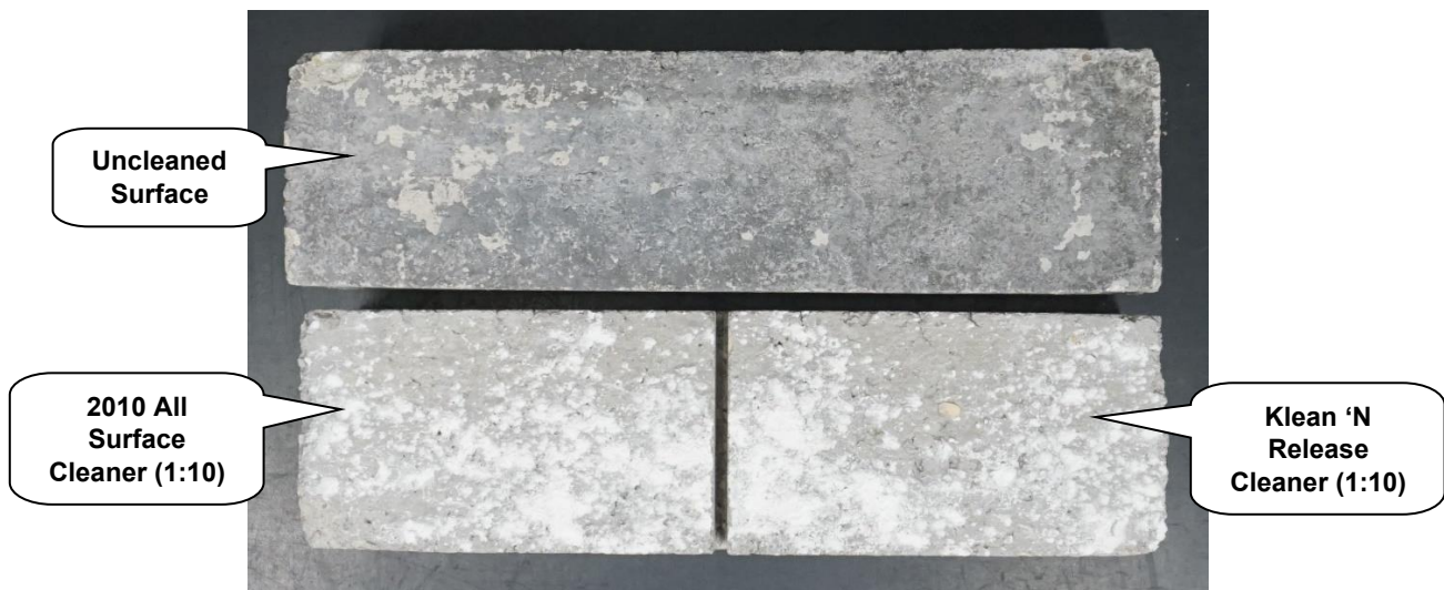
"Gettysburg" Concrete Brick After Cleaning
