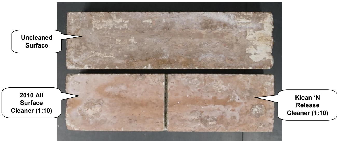
"Majestic" Concrete Brick After Cleaning
